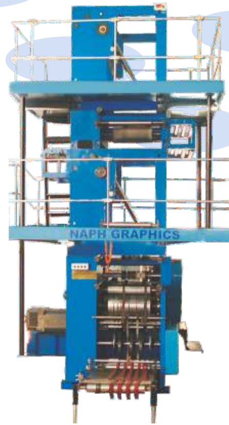
Balloon (Upper) Former for on line Supplement insertion
